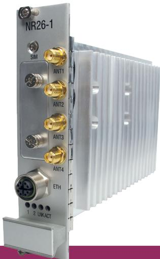
The further development of railway communication towards the FRMCS system is progressing rapidly. As a decisive step in this process, Funkwerk has developed a plug-in card for the MESA26 train radio system. This card enables seamless communication in public and private 4G/5G radio networks and is equipped with a self-sufficient processor unit and a project-specific, exchangeable 4G/5G modem. It also enables further data processing, for example to offer a state-of-the-art MCX service.
