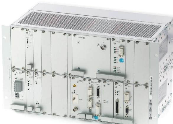
The MTRS 1+A RSH is a terminal unit for the purpose of train radio, shunting radio and data applications which operates in GSM-R networks and in the analogue radio networks in accordance with UIC 751-3 (450 MHz). It fulfils the European requirements for use in rail vehicles.
