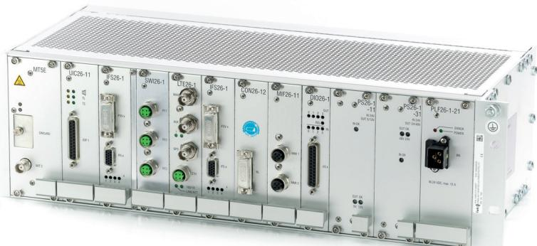
The CR26 central unit is a train radio for GSM-R radio networks and ensures the operational communication of the train driver. The CR26 can be extended with an ARM26/ARM26C analog radio to a dual-mode train radio for voice radio/shunting radio and data radio applications.
