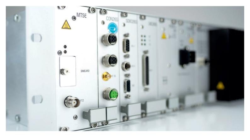
The Cabradio **CR26S** is a terminal unit for the purpose of train radio, shunting radio and data applications which operates in GSM-R networks and in the analogue radio networks. It fulfils the European requirements for use in rail vehicles. The device has a modular design and can therefore be configured according to the respective customer requirements.
