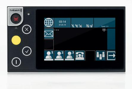
Based on the experience of many years in the field of train radio, Funkwerk has developed a 5G-based cab radio. The compact next-generation cab radio is used in modern mobile and railway communication systems (5G / FRMCS).
