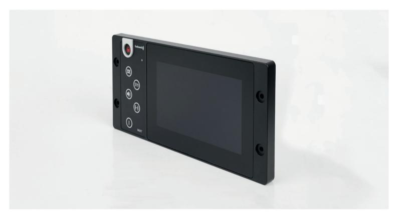
The operating device **MMIT** as part of the train radio system **MESA®26** is designed for the menu-driven operation of digital and analogue train radio. It fulfils the requirements for the operation on rail-vehicles and it is designed for the console installation in the driver's cabin. With the use of handset and a loudspeaker the driving crew is able to carry out diverse communication tasks.
