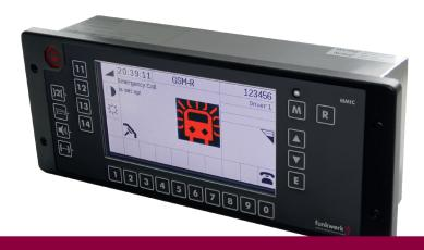
The operating device MMIC as part of the train radio system MESA 26 is designed for the menu-driven operation of digital and analogue train radio. It fulfils the requirements for the operation on rail-vehicles and it is designed for the console installation in the driver's cabin. The driving crew is able to carry out divers communication tasks with this MMIC in combination with a handset and a cabin loudspeaker.
