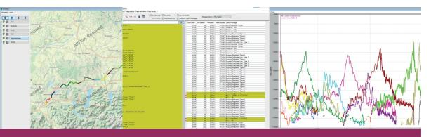
Trace2 can be used to display and analyze recorded trace messages. The trace data are created on the MT module and are transferred via a proprietary binary trace protocol between the MT module and PC to the Trace2 server where they are decoded.
