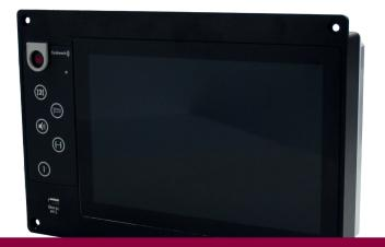
The operating device MMIL as part of the train radio system MESA 26 is designed for the menu-driven operation of digital and analogue train radio. It fulfils the requirements for the operation on rail-vehicles and it is designed for the console installation in the driver's cabin. With the use of handset and a loudspeaker the driving crew is able to carry out diverse communication tasks. It can be equipped optionally with a handsfree system featuring echo compensation and noise cancelling.
