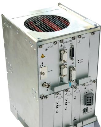
The MTRS 1 RI is a terminal unit for the purpose of train radio, shunting radio and data applications which operates in GSM-R networks. It fulfills the European requirements for use in rail vehicles.
