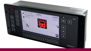
The operating device MMIL as part of the train radio system MESA 26 is designed for the menu-driven operation of digital and analogue train radio. It fulfils the requirements for the operation on rail-vehicles and it is designed for the console installation in the driver's cabin. The driving crew is able to carry out divers communication tasks with this MMIC in combination with a handset and a cabin loudspeaker.
