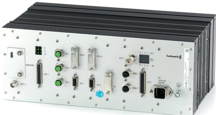
The CR26P central unit is a train radio for GSM-R radio networks and ensures operational communication for the train driver. The CR26P can be expanded with an ARM26P/x analog radio to form a dual-mode train radio for voice radio/shunting radio and data radio applications. The CR26P complies with protection class IP54.
